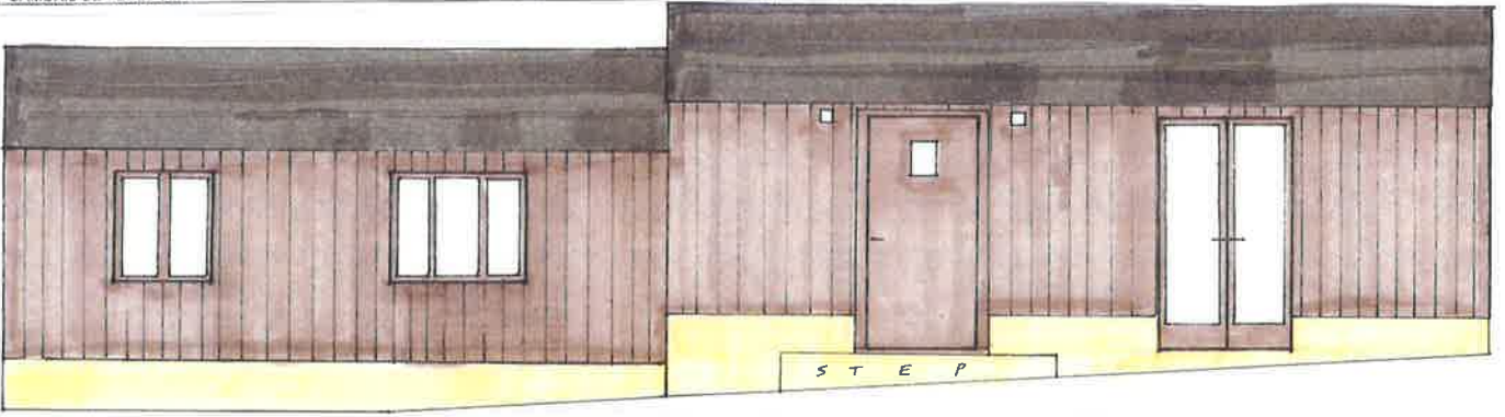
FRONT ELEVATION - EAST - SHOWING SITTING ROOM WINDOWS, ENTRANCE DOOR WITH EXTERIOR DOWNLIGHTS, PATIO DOORS.
